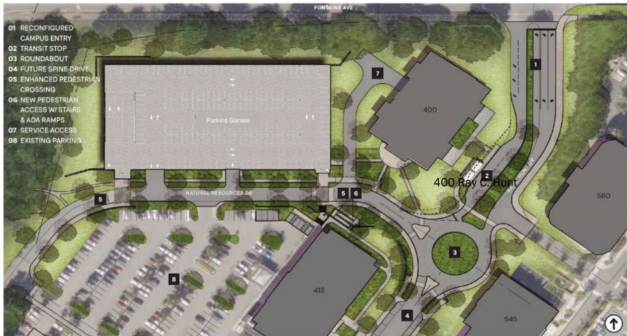
Plan view of the proposed site for the entry road, roundabout, transit stop, central spine road, and parking garage
